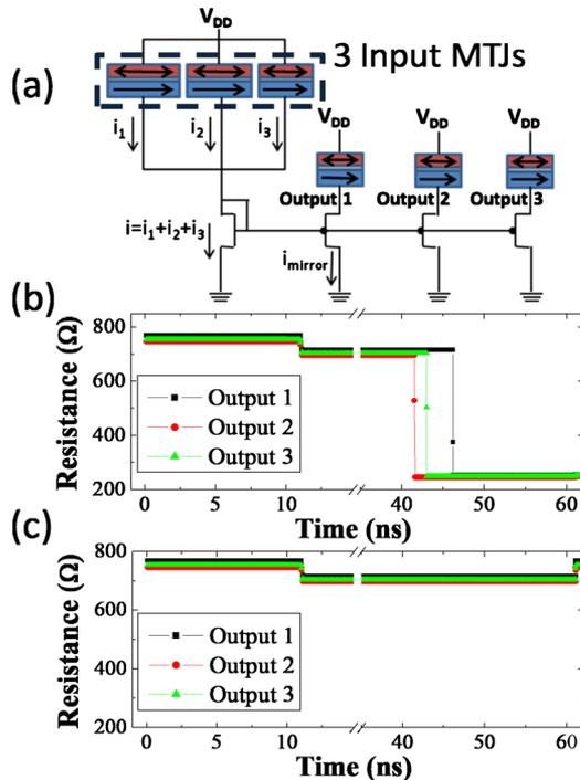
FIG. 3. (Color online) (a) Schematic of the MTJ logic and CMOS current mirror circuit and majority gate simulation results showing fan-out to three different MTJ outputs using CMOS for (b) 100 and (c) 110 input states.
