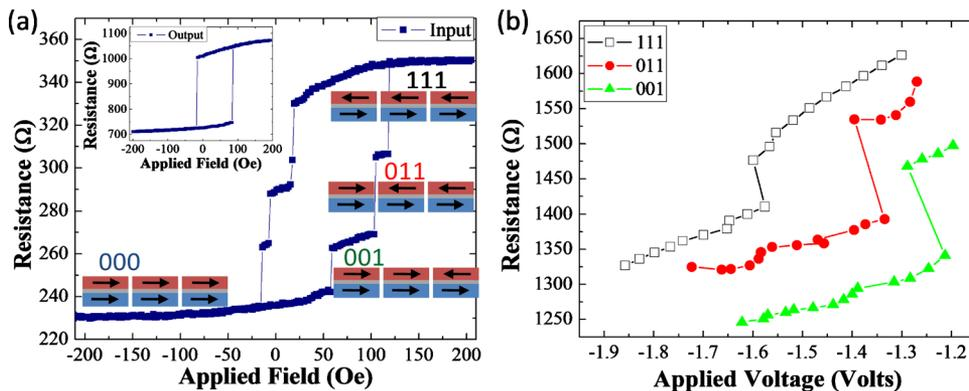
FIG. 2. (Color online) (a) Field switching loop of the input with the different resistance states defined as logic states. (Inset shows output MR loop) and (b) current switching of the output MTJ for three different resistance states of the input.
