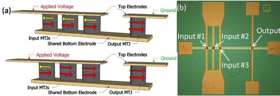
FIG. 1. (Color online) (a) Working principle of the circuit with three MTJs connected in parallel to form the input and connected in series with the output to form the voltage divider circuit, (b) optical image of the top view of the fabricated device.
